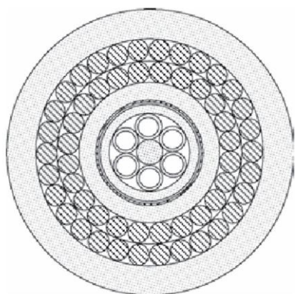
Figure 2 Double-layer Steel Wire Armor Climbing Direct Burial Optical Cable
