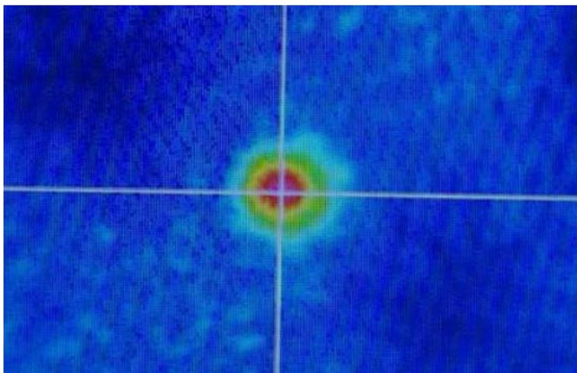
Figure 4. Optical Field Distribution
