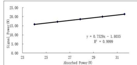
Figure 2. 915nm Pump Light Conversion Efficiency Test Results
