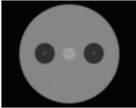
Figure 1. End View of Polarization-maintaining Yb-doped Fibre
